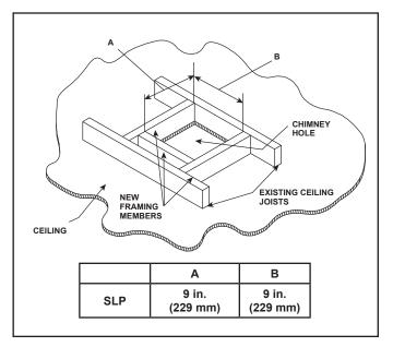
Figure 10.14 Hole and New Framing Members
